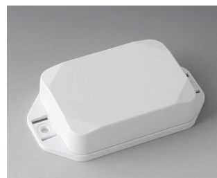
B1824227 MINI-DATA-BOX EF50, high, with flanges ASA+PC (UL 94 V-0) traffic white RAL 9016 2.76"x1.97"x0.79" IP 65 opt., IP 40
