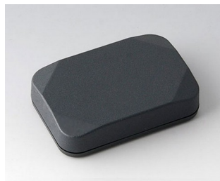
B1822118 MINI-DATA-BOX E40, flat ASA+PC (UL 94 V-0) anthracite gray RAL 7016 2.36"x1.57"x0.59" IP 65 opt., IP 40
