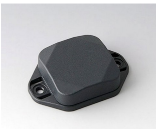
B1802128 MINI-DATA-BOX SF40, flat, with flanges ASA+PC (UL 94 V-0) anthracite gray RAL 7016 1.57"x1.57"x0.59" IP 65 opt., IP 40
