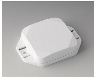
B1804127 MINI-DATA-BOX SF50, flat, with flanges ASA+PC (UL 94 V-0) traffic white RAL 9016 1.97"x1.97"x0.59" IP 65 opt., IP 40
