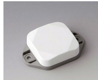
B1802126 MINI-DATA-BOX SF40, flat, with flanges ASA+PC (UL 94 V-0) traffic white RAL 9016 1.57"x1.57"x0.59" IP 65 opt., IP 40
