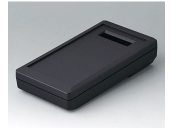
A9073319 DATEC-MOBIL-BOX S, Vers. III ABS (UL 94 HB) black RAL 9005 5.98"x3.27"x1.32" IP 65 opt.
