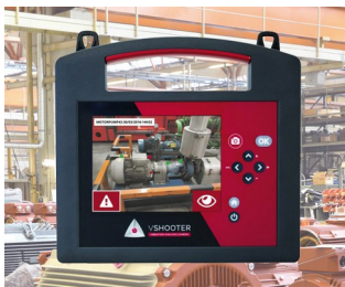
Diagnostic camera for illustrating the machine status
