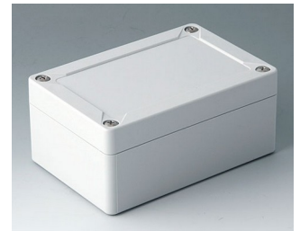
C7012011 IN-BOX ABS (UL 94 HB) light gray RAL 7035 4.80"x3.23"x2.17" IP 66, IP 67, IK 07
