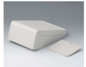
B4056337 UNITEC M, 0.02/0.06 ABS (UL 94 HB) off-white RAL 9002 5.83"x8.27"x3.15" IP 40
