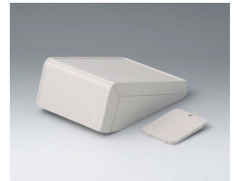
B4054237 UNITEC S, 0.02/0.06 ABS (UL 94 HB) off-white RAL 9002 4.92"x6.97"x2.72" IP 40
