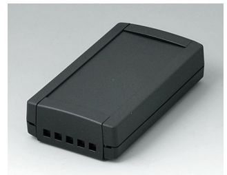
B1055469 TOPTEC 123 F, Vers. II ABS (UL 94 HB) black RAL 9005 4.84"x2.68"x1.18" IP 40
