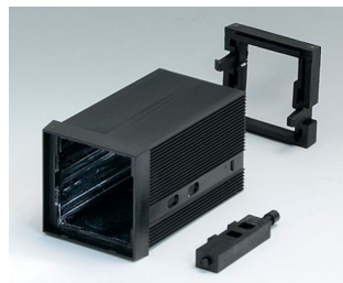
B6012021 DIN-MODULAR CASE TYPE A PPO (UL 94 V-0) black RAL 9005 1.89"x1.89"x2.95"
