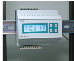
Power measuring device for energy analysis
