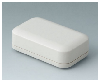
A9403107 EVOTEC 80, Vers. I ASA+PC (UL 94 V-0) off-white RAL 9002 3.15"x1.97"x1.02" IP 65 opt., IP 40
