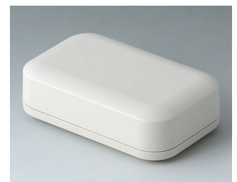
A9423107 EVOTEC 100, Vers. I ASA+PC (UL 94 V-0) off-white RAL 9002 3.94"x2.44"x1.22" IP 65 opt., IP 40
